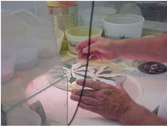
Photo #4 – The application of colored powders has been completed and the final glass plate is applied on top to complete the sandwich. This actually becomes the bottom of the plate as it will be flipped before being placed in the kiln. Firing is the next step. As you can see the process is very labor intensive and time consuming.
